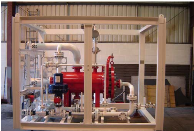
ConocoPhillips Ekofisk 2/4J – 340,000 BPD Deoiling Hydrocyclone Package
