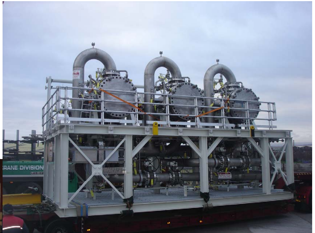
ConocoPhillips Ekofisk 2/4J – 340,000 BPD Deoiling Hydrocyclone Package
