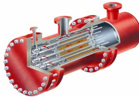
Figure 6 – Conventional Deoiling Hydrocyclone vessel
