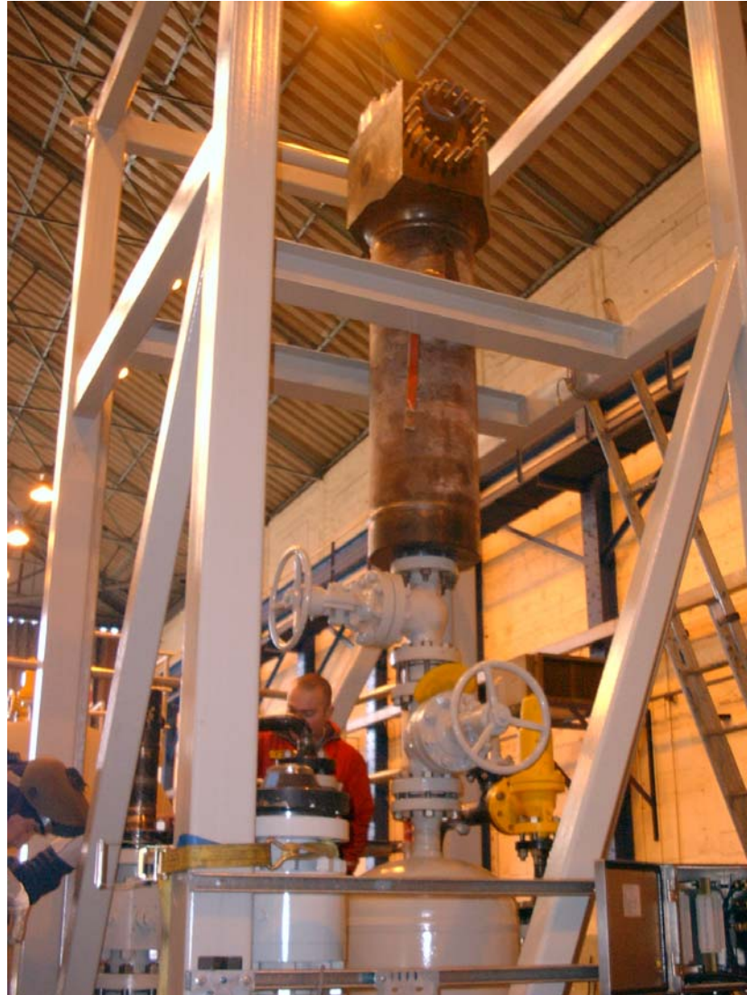
Fig. 3 – Typical Cyclotech WDC System with upper cyclone vessel and lower accumulator vessel
